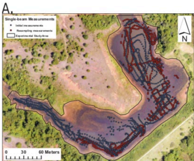
Figure 6. Bathymetry of Finn Creek 21 Reservoir using the single-beam echosounder. (a) Cumulative sampling points taken with the single-beam echosounder during August of 2017. (b) Bathymetric mapping built with the single-beam echosounder is shown.
