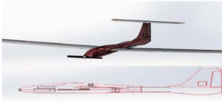
Figure 4. Tempest UAS illustrating location of LDCR and MiCo antenna elements.
